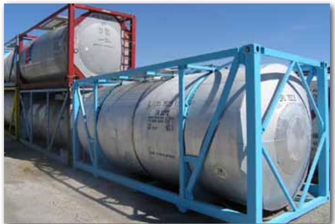
Heresite lining protects iso-tanks from harsh chemicals.
